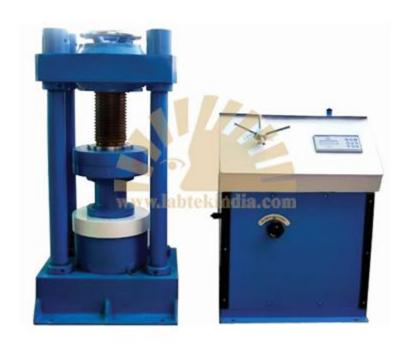
Compression Testing Equipment Electrically cum Manually (Hand) Operated. The loads are measured on Bourdon tube type load gauges which are calibrated against certified proving rings. The load gauges are fitted with a maximum load pointer.
